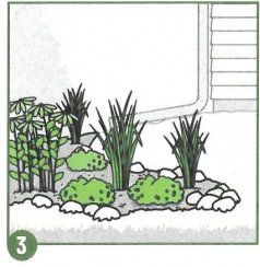
3 Install a rain garden to collect stormwater (at least 5 m from the foundation).
